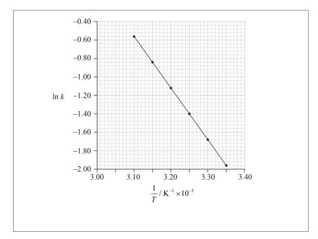
Using data from the graph, determine the activation energy,  $E_{\rm a}$ , correct to **three** significant figures and **state its units**. [4]
